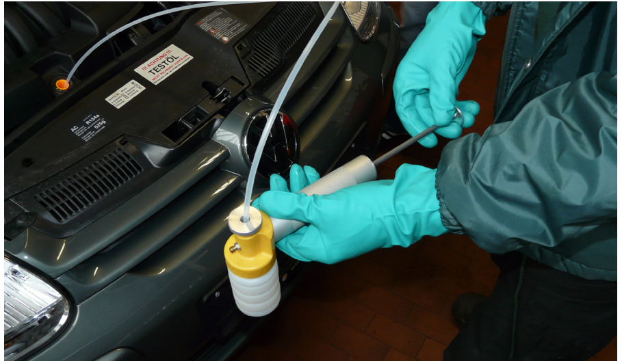
Drawing an oil sample for testing
